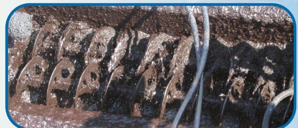
Automatic mixing process is continuously monitored by trained operators. Other staff cleans the surface before slurry application, closes the working site to the traffic, controls the suitability of layout process, cleans the metal manhole cover after the application and completes the slurry mortar layout process where the layout
